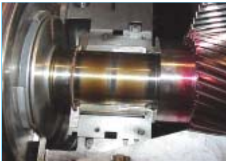
Fig 2 - Brown varnish on journals and shaft
